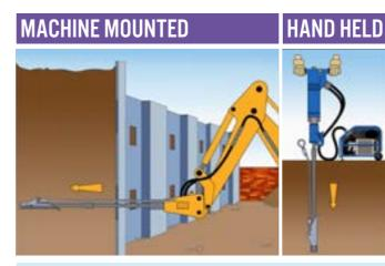
Vulcan anchors are designed to be driven into the ground using hydraulic or percussion equipment, with little or no disruption to the structure or surrounding area.
