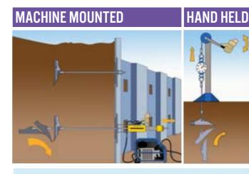
A tensile load is applied to the attached tie bar or tendon. This rotates the anchor into the locked position for maximum load holding capacity. The anchor is then proof tested to the designed loading requirements before the top termination is fitted, as specified by the civil or structural engineer.
