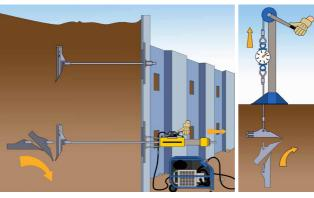
A tensile load is applied to the attached tie bar or tendon. This rotates the anchor into the locked position for maximum load holding capacity. The anchor is then proof tested to the designed loading requirements before the top termination is fitted, as specified by the civil or structural engineer.
