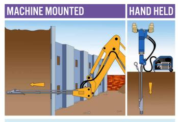
Vulcan anchors are designed to be driven into the ground using hydraulic or percussion equipment, with little or no disruption to the structure or surrounding area.
