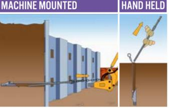
Once the anchor has been driven to the required depth the drive rod is removed for reuse.
